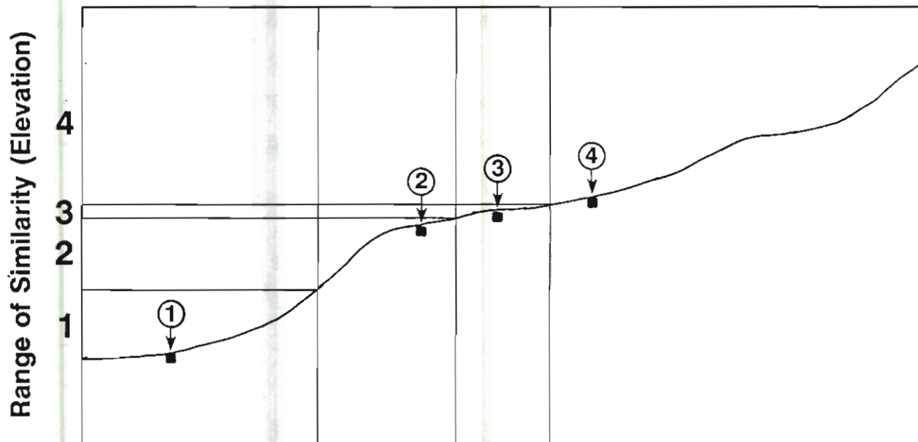
Fig. 1. A diagram to show the possible conflict in the climate comparison map. Four comparison points are shown on an elevation profile. The profile is divided between them by allocating the points all the areas closest in elevation. 4 captures all the high ground, 1 all the low ground and 3 is caught in between 2 and 4.
